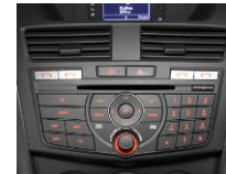
Factory Audio Unit (AHU)
