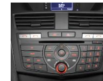
Factory Audio Unit (AHU)
