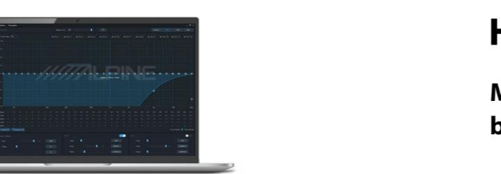
The PXE-X121-12EV is designed with user convenience in mind. By using the companion mobile app or PC software, users can quickly and easily configure parameters such as equalisation curves, phase and gain levels, time delays and crossover points for precision sound customisation.
